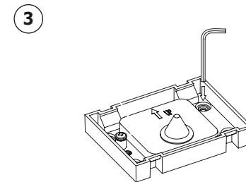
Cut a part of the bushing, but ensure it's smaller than the cable diameter
