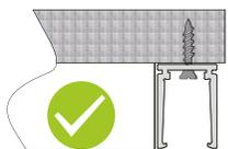
Install the screw into position and ensure the screw head is flush or lower the base of aluminum profile.
