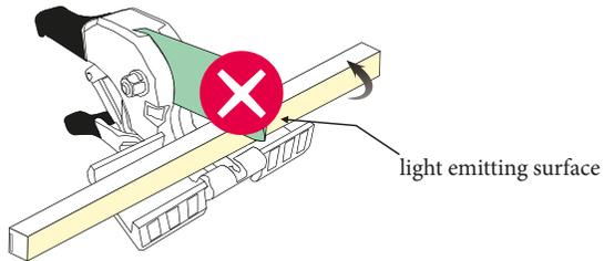
Place the LED strip and cut to the circuit board in a lying shape.
