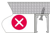
Gradient installing of screw.
