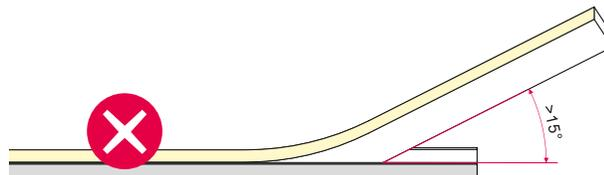
The circuit board could be damaged if installing angle larger than 15 degree.
