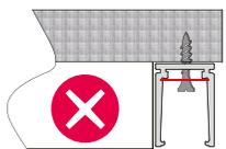
Screw head above to the base of aluminum profile.
